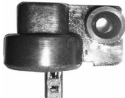
The rollover sensor, also known as a "banking" sensor, is a safety feature. If the banking angle of the motorcycle goes below 60° OR in the event of an accident causing the motorcycle to fall over on either of its sides with the engine running, the rollover sensor will "command" the ECU to cut off both the fuel supply and ignition, thus stalling the engine to prevent any further damage from being caused by the engine that may be running with a stuck open throttle and the gears engaged.
