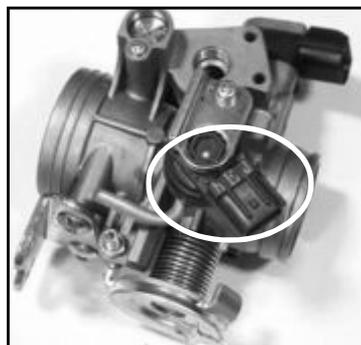
The MAP sensor monitors the manifold pressure at the intake end and provides data to the ECU on a real time basis. This helps the ECU to calculate the air density and the air inflow rate and determines the fuel injector opening duration to provide the required amount of vaporized fuel into the combustion chamber for optimum performance of the motorcycle.
