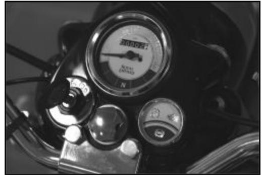
When both the Ignition & Engine kill switch is "ON" and after vehicle is started, MIL will glow for few seconds and switch OFF, this indicates that all the functions of EMS are functioning correctly.
