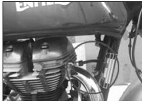
It detects residual oxygen in the exhaust gases versus the amount of oxygen in the atmosphere and provides the data on a real time basis to the ECU based on which the fuel injection is metered continuously to control exhaust emissions and for optimum performance of the motorcycle.
