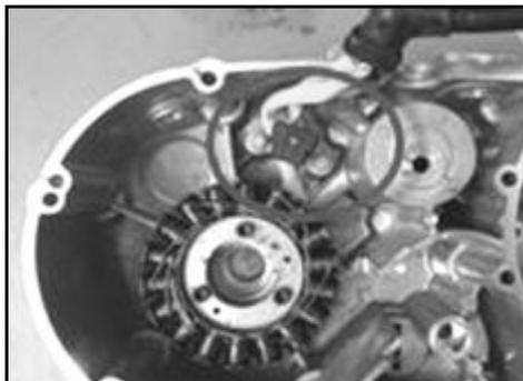
It provides an alternating electrical pulse to the ECU, to determine crankshaft speed and TDC position by scanning the 17 pips and 1 long gap between 2 particular pips on the rotor. This input helps the ECU to optimize both fuel injection as well as Ignition advance required to suit the crankshaft rotation speed (RPM).
