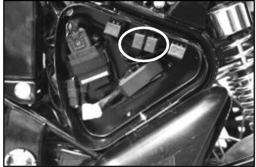
The EFI ECU Power relay supports functioning of the ECU and fuel pump. The Side stand relay provides the inputs regarding the position of the side stand to the ECU. In the event the side stand is NOT retracted and the motorcycle is attempted to be started, it signals the ECU which cuts off the fuel supply thus preventing the engine from starting.
